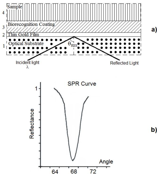
Fig. 1. (a) The multilayer SPR biosensor structure showing all elements, where the SPR curve (b) results from resonant absorption of an incoming light beam at the dielectric-metal interface under specific boundary conditions.
