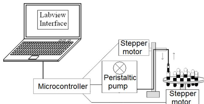
Fig. 2. The autosampler set-up with all elements connected to a microcontroller and a PC, which is used for programming and user interface.
