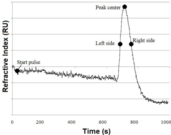
Fig. 4. The sensorgram used for the calculation of the molar diffusivity at the 5% ethanol-water solution.
