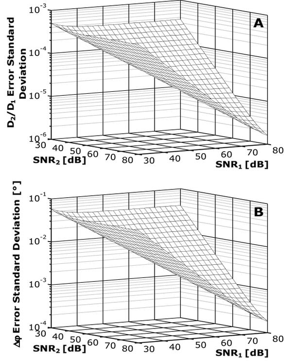
Fig. 3. Standard deviation of the amplitude ratio (A) and phase difference error (B) for the seven parameter sine fit algorithm as a function of the two signal to noise ratios for  $D_1=1$  V and  $D_2=0.5$  V.
