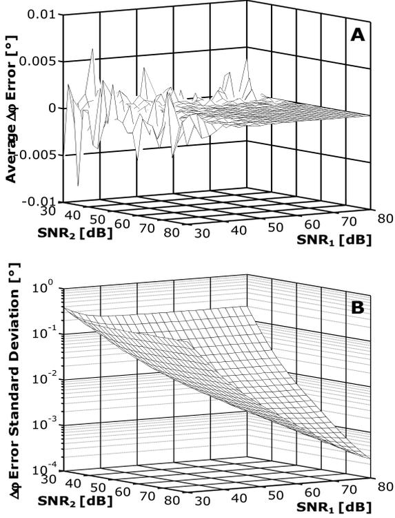
Fig. 2. Average phase difference error (A) and corresponding standard deviation (B) for the ellipse fit algorithm as a function of the two signal to noise ratios for  $D_1=1$  V and  $D_2=0.5$  V.
