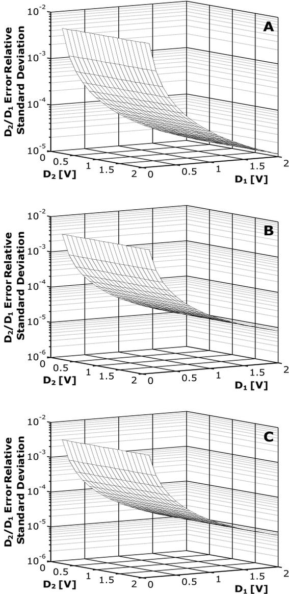
Fig. 5. Relative standard deviation of the amplitude ratio for the ellipse fit (A), seven parameter sine fit (B) and spectral sinc fit (C) as a function of the two signal amplitudes for  $SNR_1=SNR_2=60$  dB.
