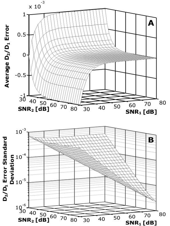
Fig. 1. Average amplitude ratio error (A) and corresponding standard deviation (B) for the ellipse fit algorithm as a function of the two signal to noise ratios for  $D_1=1$  V and  $D_2=0.5$  V.
