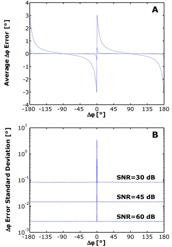
Fig. 6. Average phase difference error (A) and standard deviation (B) for the ellipse fit algorithm as a function of the phase difference and common SNR for  $D_1=1$  V and  $D_2=0.5$  V.
