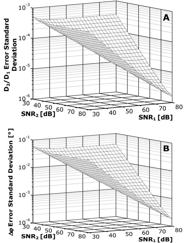
Fig. 4. Standard deviation of the amplitude ratio (A) and phase difference error (B) for the spectral sinc fit algorithm as a function of the two signal to noise ratios for  $D_1=1$  V and  $D_2=0.5$  V.
