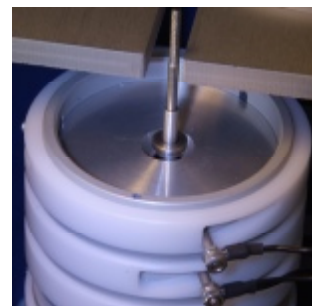
Fig. 4. Handling system for the weights: 1 g disc weight on the suspension system lifted by the aluminium disc and the white lifting mechanism with the contact control
