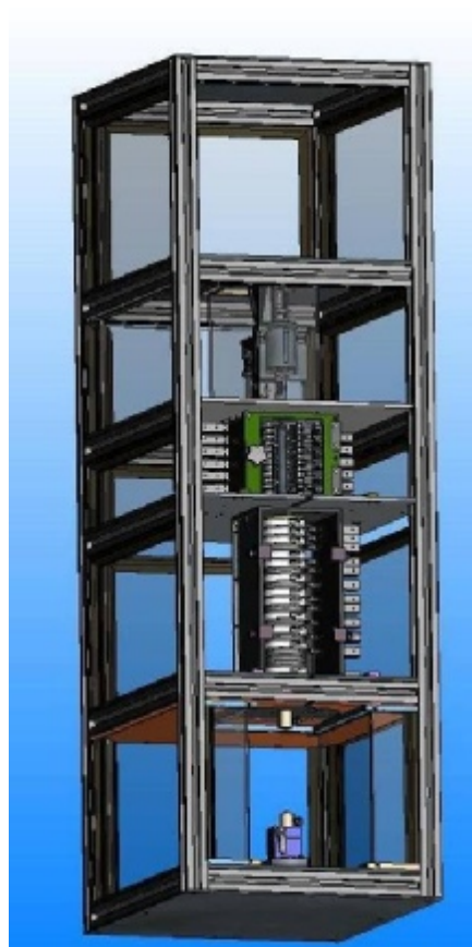
Fig. 1. Concept and Construction of the 10 N Dead Load Machine
