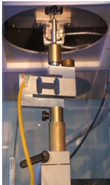
Fig. 10. The rebuilt 300 g balance as a standard force transducer connected to the suspension system of the balance. Above the force transducer there is a clamp to fix the suspension system
