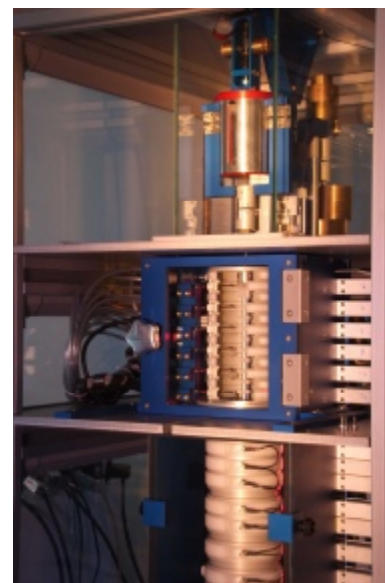
Fig. 5. Handling system for the weights of the 10 N Dead Load Machine
