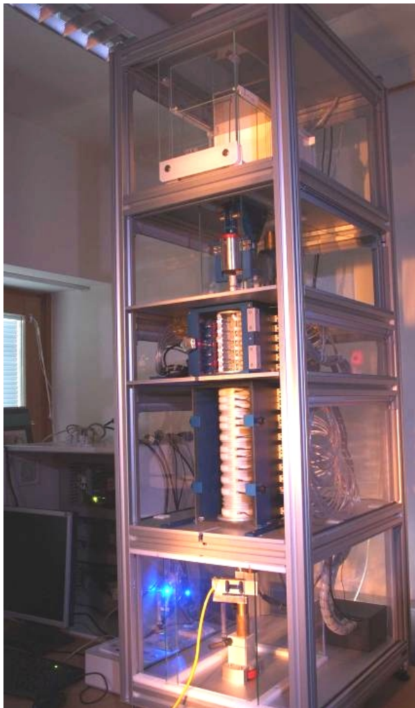
Fig. 2. realisation of the 10 N Dead Load Machine (without covering); mechanism for the wire weights and for the disc weights in the middle; in the lower ground is the measurement cell for the standard force transducer, on the top the balance
