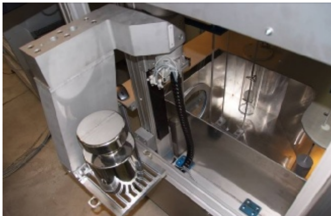
Fig. 8. Load alternator (lift system) for the 50 kg test weight in the liquid tank; in the background there is the measurement chamber for the liquid density determination; on the right there is the additional sinker for liquid surface motion compensation.
