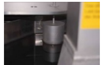
Fig. 7.; the sinker to compensate the liquid surface motion caused by the movement of the lift in the foreground
