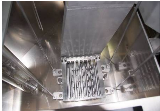
Fig. 3. Load alternator and suspension system for the test weight in the liquid tank; on the left the measurement chamber for the liquid density determination can be seen
