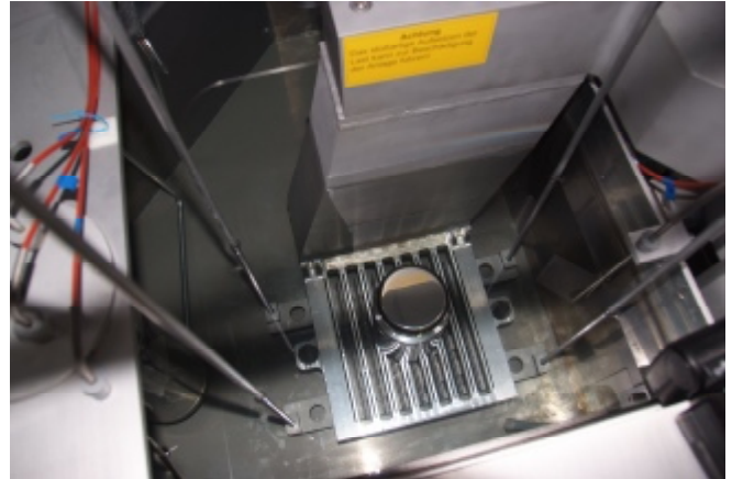
Fig. 5 and 6: Load alternator for bringing in a 10 kg test weight in the liquid tank; on the left there is the measurement chamber for the liquid density determination also with the load alternator; the red wires shows the platinum resistance sensors for the temperature measurement in the chamber of the liquid density measurement and these of the liquid tank
