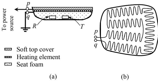
Fig. 2. A cross-sectional view (a) and top view (b) of the sitting area of the seat with integrated heating elements.
