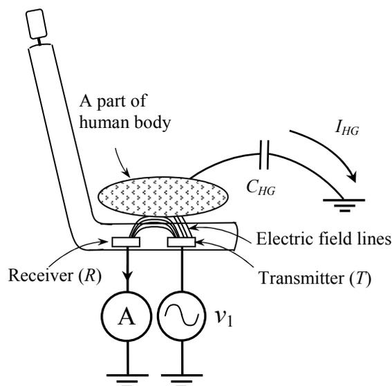
Fig. 1. Principle of seat occupancy detection based on electric field shielding. Parts of the electric field lines from the transmitter to the receiver are shielded by the human body.  $C_{HG}$  is the equivalent value of distributed capacitances between the human body and ground. 'A' indicates a low impedance shunt.
