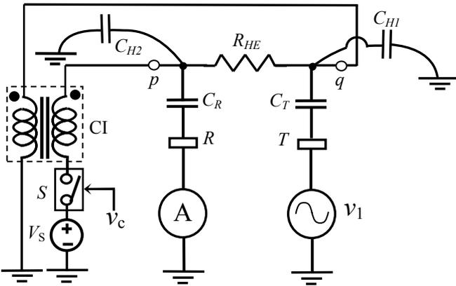
Fig. 4. Equivalent electrical circuit of the system.  $R_{HE}$  is the resistance of the heating element.  $C_{H1}$  and  $C_{H2}$  represent the distributed capacitances between the heating element and ground.
