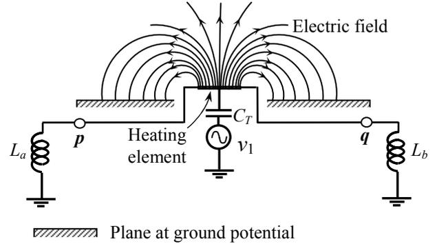
Fig. 3. Heating element of the seat connected to ground through inductors  $L_a$  and  $L_b$ . The heating element will be at a certain potential, due to the sinusoidal source  $v_1$ , and the coupling capacitance  $C_T$ . A pictorial view of the electric field is also shown
