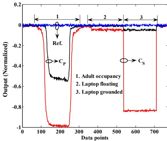
Fig. 8. Output signal obtained for conditions such as an adult occupancy, laptop floating and laptop grounded conditions respectively. The measurement result at  $f_r$  (1.5 MHz) is indicated by  $C_S$  and that at 0.5 MHz is marked by  $C_P$ .
