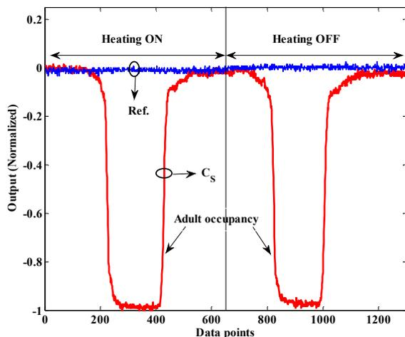
Fig. 7. Output signals recorded for an adult occupancy, when the heating element was turned ON (left side) and turned OFF (right side) conditions.  $C_S$  indicates the output from the sensor at resonance frequency. The reading corresponding to a vacant condition is shown by a reference (Ref.) signal.
