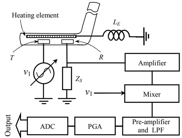
Fig. 6. Block diagram representation of the measurement setup. During the investigations, the heating element was powered from a dc source  $V_S = 12$  V.
