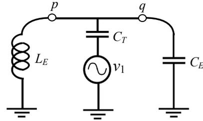
Fig. 5. Simplified electrical equivalent circuit showing the resonance condition. Capacitance  $C_E$  is the parallel combination of  $C_{H1}$ ,  $C_{H2}$  and  $C_R$ .  $L_E$  is the effective inductance offered by the coupled inductor (CI) to a common mode signal.
