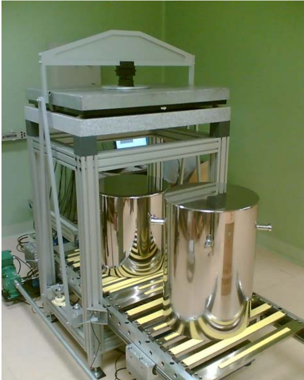
Fig 5. Weight handler system general view
