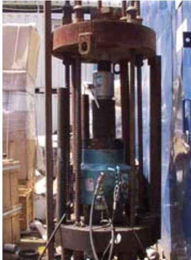
Fig. 6. Loading and measuring in vertical closed frame.
