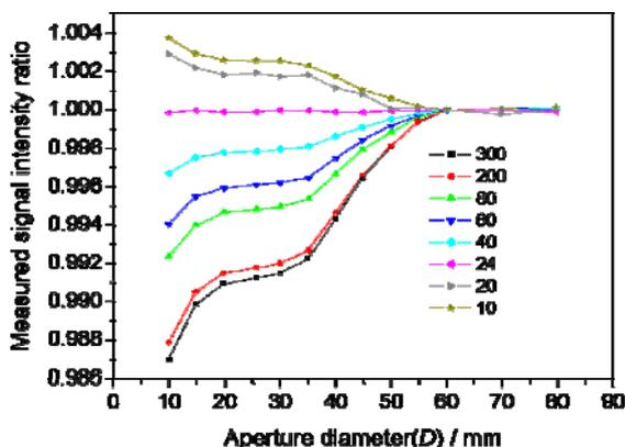
Fig. 2. Normalized TRT signal intensity for LT range with respect to the intensity for the aperture diameter of 60 mm.
