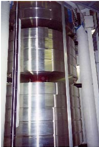
Fig. 3. Picture of large masses of Galdabini 1 MN (MCF1000).
