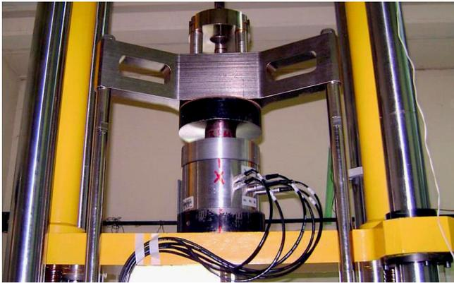
Figure 2. 160 kN six-component dynamometer.
