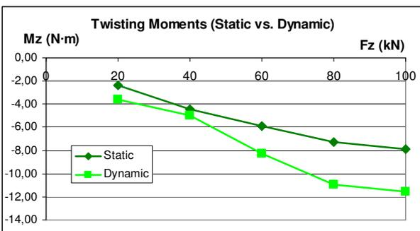
Figure 11. Twisting moments. Static vs. dynamic.
