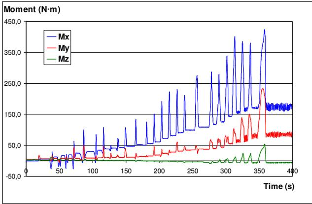
Figure 5. Bending and twisting moments. First measurement.
