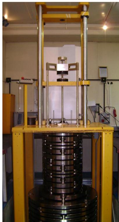
Figure 1. INTI's 110 kN primary Force Standard Machine.
