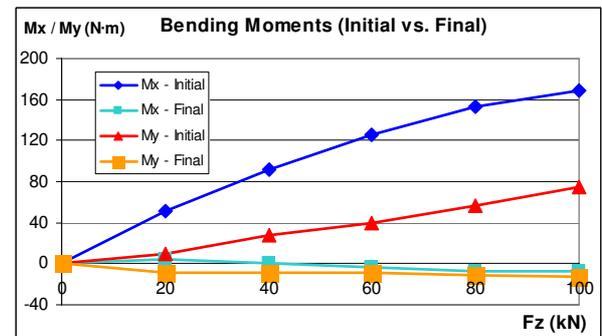
Figure 13. Bending moments. Initial vs. final mean values.
