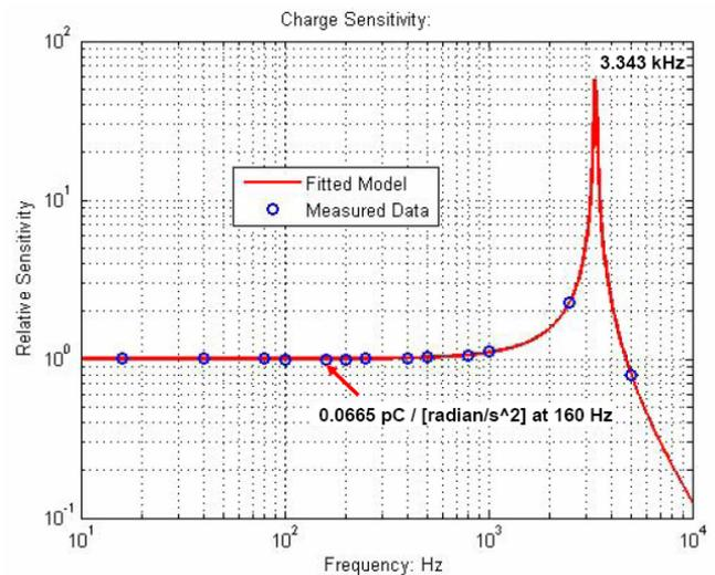
Fig.10. Measured modulus sensitivity characteristics of the first prototype angular accelerometer mad by B&K.
