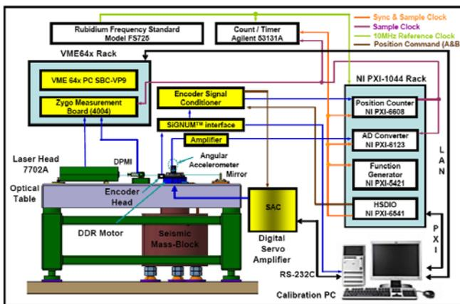
Fig.8. Configuration diagram of the primary calibration system in KRISS.
