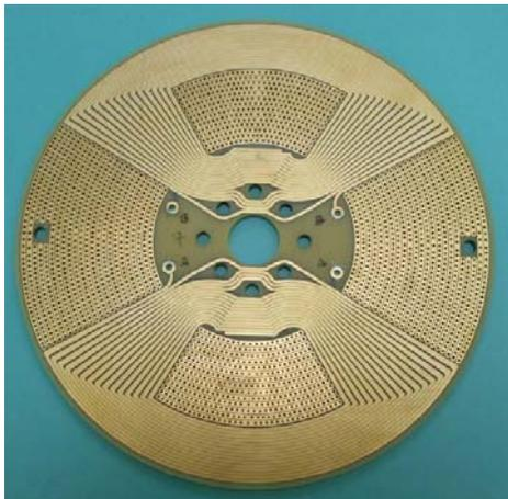
(b) 20-layer PCB-typed rotational coil.
