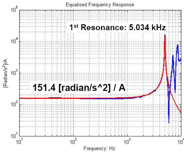
Fig.3. Frequency response of the new angular vibration exciter developed in KRISS.
