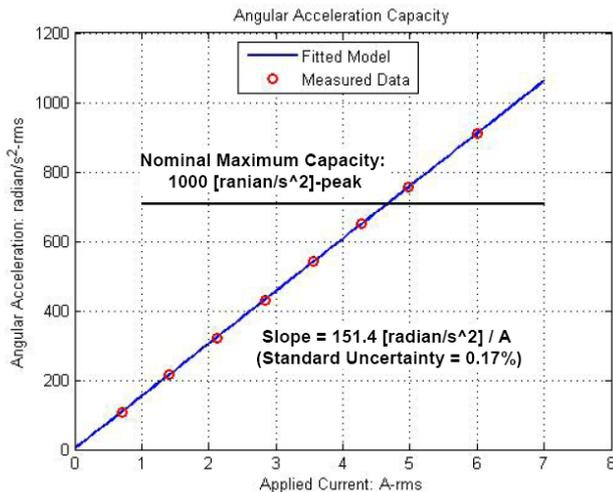
Fig.4. Generation capacity of angular acceleration tested at 160 Hz.
