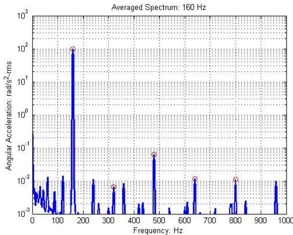
(a) Harmonic components measured at 160 Hz.
