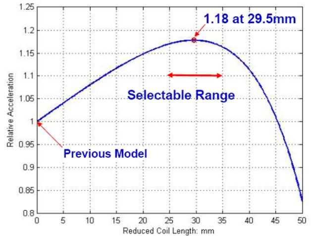
Fig.2. Normalised angular acceleration level in reduction of the effective coil length.
