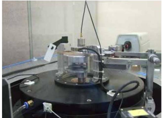
Fig.9. Photo of the first prototype angular accelerometer fixed on the upper surface of the angle prism holder.
