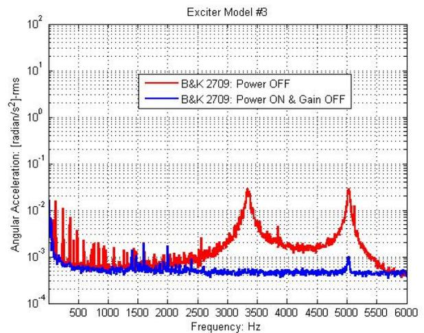
Fig.5. Background vibration levels measured from the high-precision ball-bearing supported angular vibration exciter.
