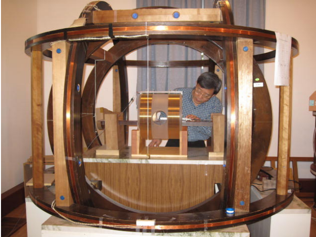
Fig. 5. Photograph of coil constant measurement.
