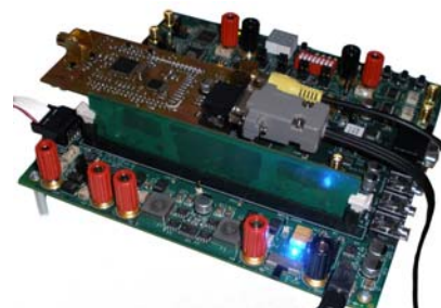
Fig. 4. Custom extension video I/O board with SANTA CRUZ connector developed in [15] attached to the standard Altera video development kit.
