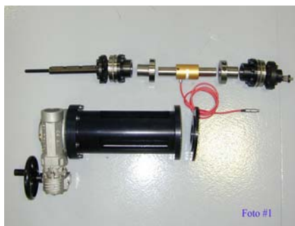
Fig. 1. Calibration bell and its components (Serial 031): specific equipment for the calibration of torque transducers mounted on Atlas Copco BLM JSB benches by the use of reference transducers.
