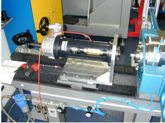
Fig. 4. Calibration bell mounted on first line calibration bench using the special adaptor.
