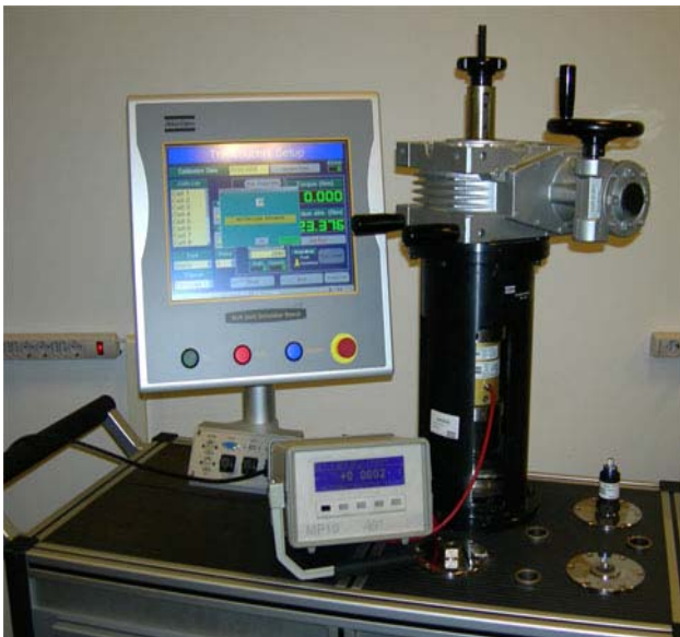
Fig. 6. Calibration bell 2000 mounted on a bench for calibration
