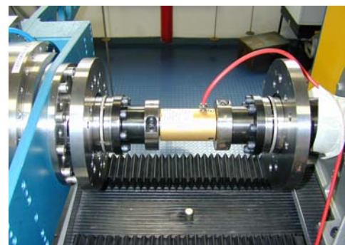
Fig. 3. The transducer mounted directly on first line calibration bench, using the joints and adapters of the bell.
