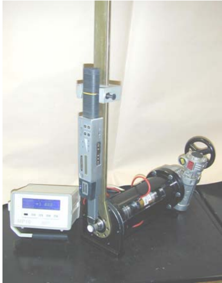
Fig. 8. Calibration of torque wrench
