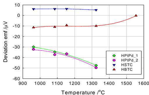
Fig.2 Deviation emf and curves for each thermocouple.
