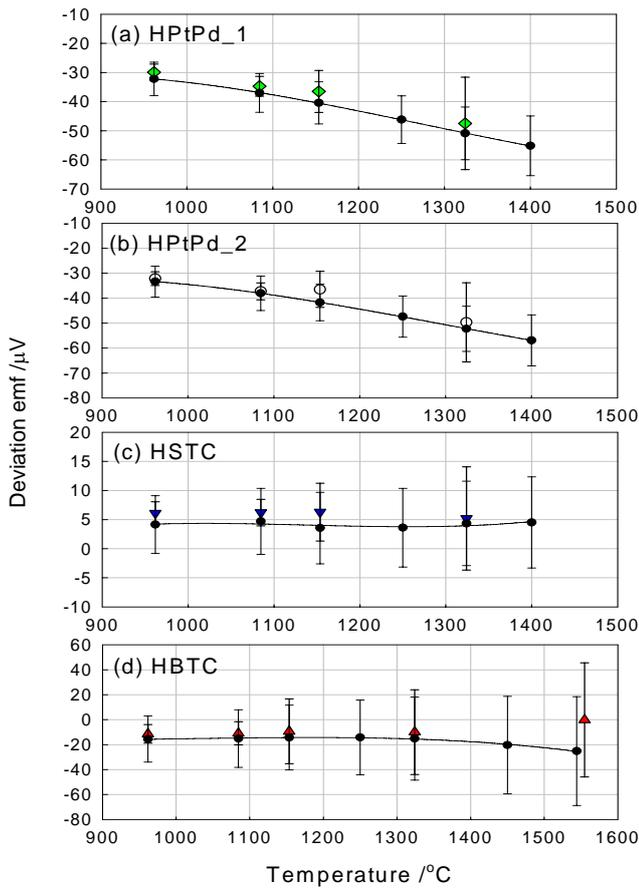
Fig.3 Variation in the deviation emf for each thermocouple. The results from the fixed-point calibrations are also shown.
