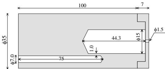
Fig. 1. A schematic diagram of the inter-comparison blackbody block. All dimensions shown are in mm.
