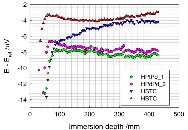
Fig. 4 Inhomogeneity results after comparison with the radiation thermometer. The terms  $E$  and  $E_{ref}$  indicate the measured and reference emf at  $180$  °C for each thermocouple, respectively.
