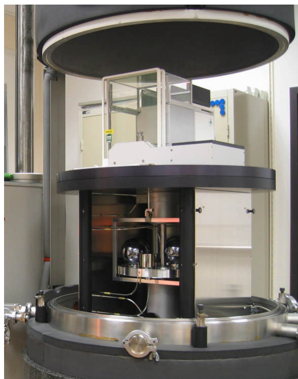
Fig. 1. Mass comparison apparatus used to check the cleaning of silicon density standards.
