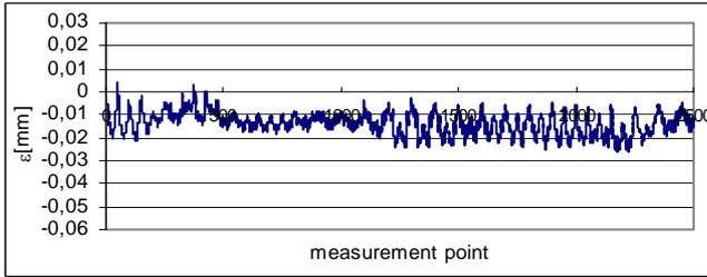
Fig. 7. Plot of geometric deviations  $\varepsilon$ ; scanning without applying radius compensation.
