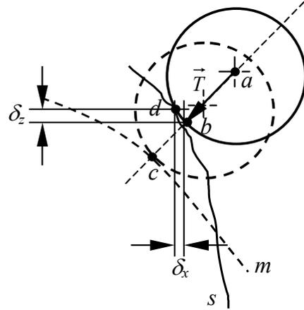
Fig. 1. Contact error: *m* – CAD model, *s* – actual surface, *a* – indicated measured point, *b* – corrected measured point, *c* – target contact point, *d* – actual contact point,  $\vec{T}$  – tip correction vector,  $\delta_x$  – error component in *X* direction,  $\delta_y$  – error component in *Y* direction.
