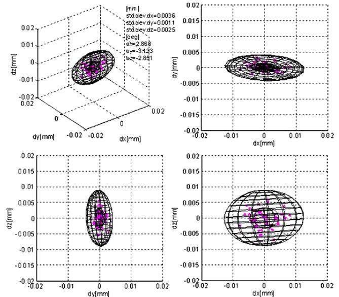
Fig. 12. Uncertainty contours and their projections on the coordinate system main planes, without compensation
