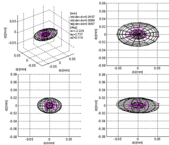
Fig. 11. Uncertainty contours and their projections on the coordinate system main planes, with applying radius compensation
