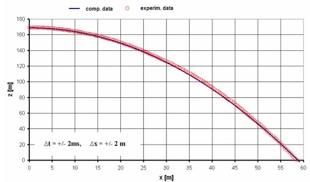
Fig. 10. Model trajectory compared with positions of the capsule registered with camera.
