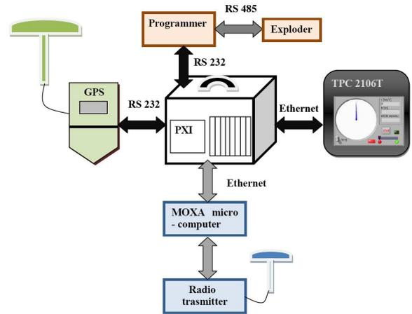
Fig. 2. A general scheme of the system of control.
