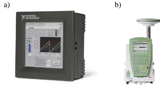
Fig. 4. Front view of the TPC - 2106T mini-computer (a). GX1230GG receiver with RX1210T controller (b).
