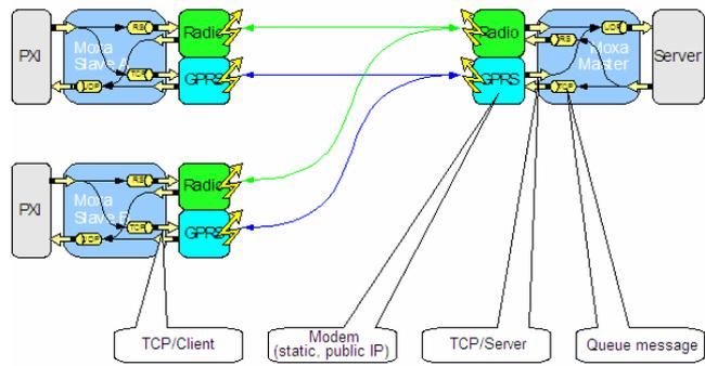
Fig. 5. Schematic view of interconnections within the system of data transmission.
