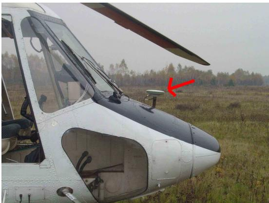
Fig. 9. The GPS antenna fixed to the nose of the helicopter.
