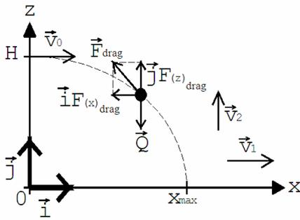
Fig. 1. Forces acting on a body falling with initial horizontal velocity.
