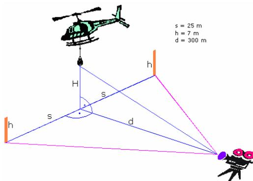
Fig. 8. Schematic view of the registration post.
