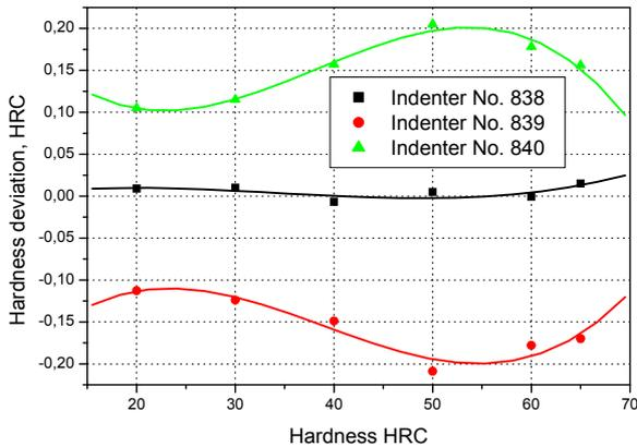
Fig. 1. Hardness deviations from the mean value of three Rockwell diamond indenters obtained for six different hardness levels.
