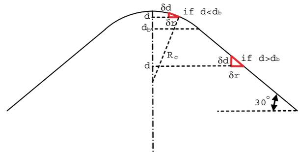
Fig. 7. Geometrical relationship between indentation depth deviation  $\delta d$  and radius deviation  $\delta r$ .
