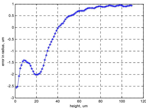
Fig. 6. Deviation between the measured and the theoretical area function curves of the Rockwell indenter No. 838.
