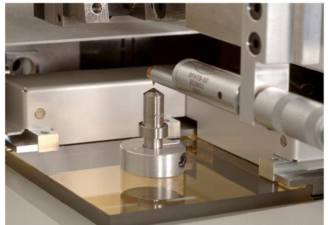
Fig. 2. Setup for the measurement of the Rockwell indenters surface with a stylus probe on the NMM. The indenter is fixed on the scanning table which is moved in 3D.
