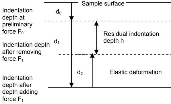
Fig. 8. Rockwell test procedure.
