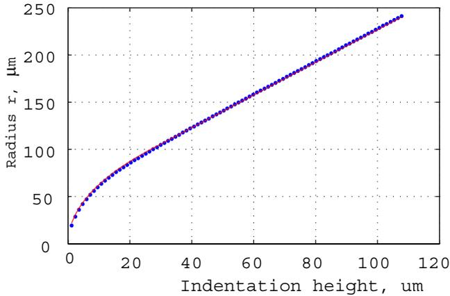
Fig. 5. Area function of a measured Rockwell indenter.
