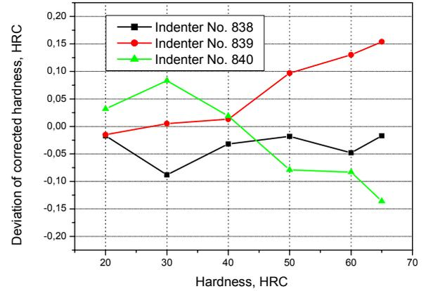
Fig. 9. Hardness deviations from the corrected hardness values of three Rockwell diamond indenters obtained for six different hardness levels.
