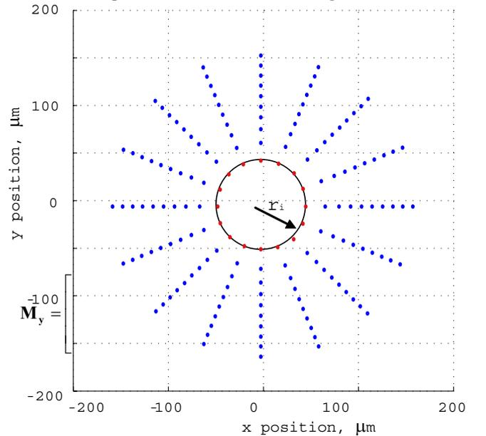
Fig. 4. Fitting the contour points having an indentation depth  $d$  to a circle. As shown by the innermost points, they are fitted by the least square method to a circle (solid line) which is the projected circle at the indentation depth  $d$ .
