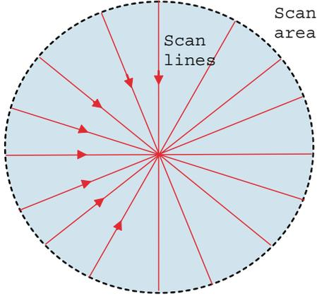
Fig. 3. Arrangement of the radial scan lines going through the apex of the indenter.
