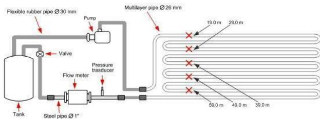
Fig.1 Experimental layout
