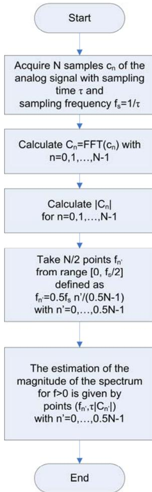
Fig.4 Developed FFT technique
