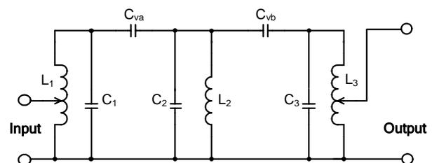
Fig. 1. Diagram of the band-pass filter
