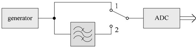
Fig. 3. Measurement setup
