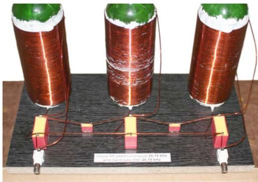
Fig. 2. Prototype of the band-pass filter
