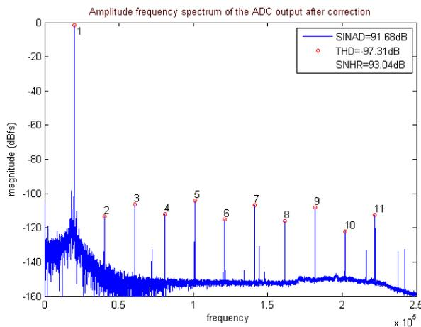
Fig. 6. Amplitude frequency spectrum computed by frequency spectrum correction method – DS 360 generator (Welch average  $100 \times 41.5$  kSa, 50% overlapping)
