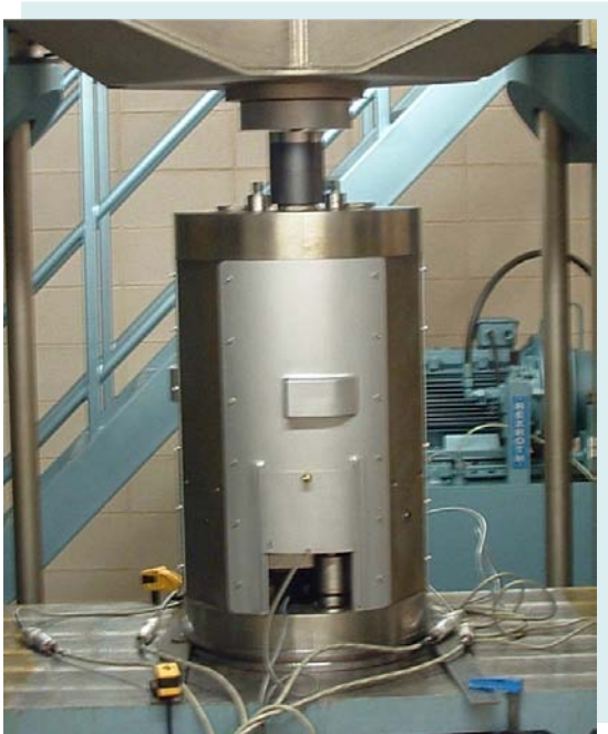
Fig. 3. The INRIM 500 kN six-component dynamometer.
