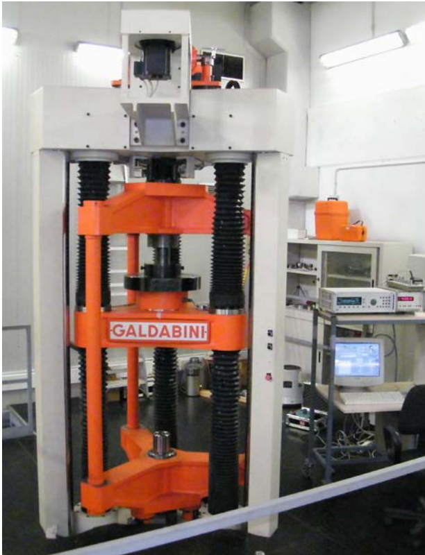
Fig. 4. The upper part of the INRIM 1 MN force standard machine.
