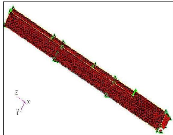
Fig. 5. Red triangular surface mesh covering the surface of the geometry.
