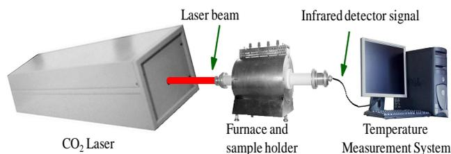
Fig. 1. Thermophysical Properties Measurement Laboratory Experimental Apparatus.
