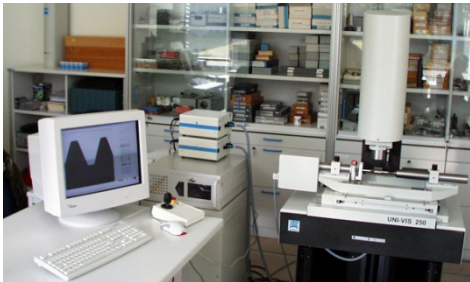
Fig.1 Example for a coordinate measuring machine, the UNI-VIS 250
