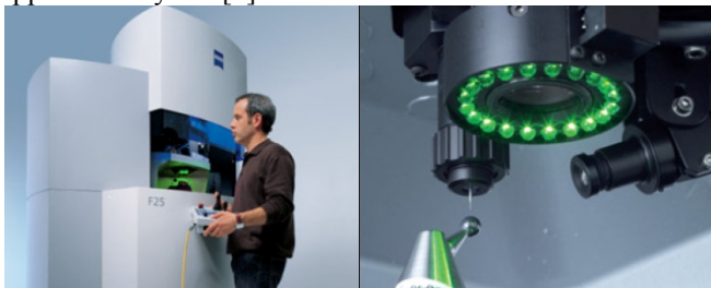
Fig. 1. Example for machine vision in a coordinate measuring machine, the Zeiss F25 [2]
