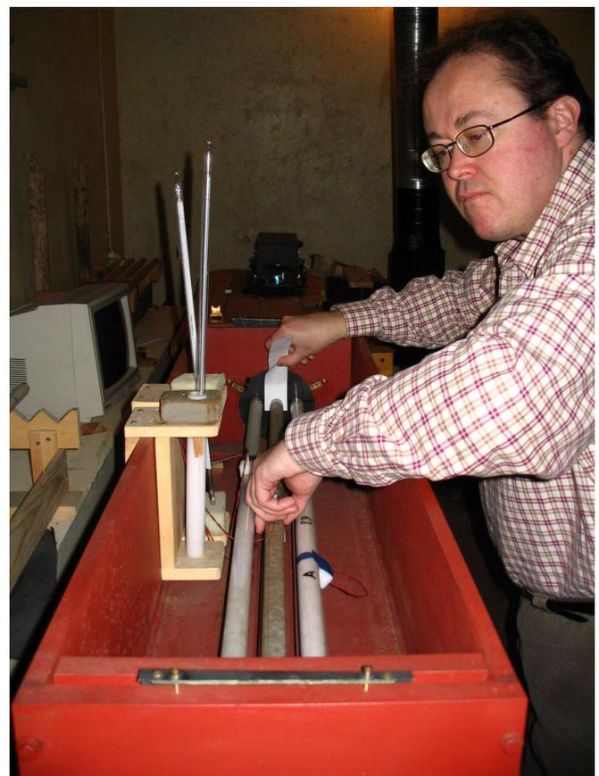
Fig. 2. Adjusting the quartz metre no. VIII for a comparison at Tuorla Observatory.
