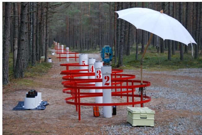
Fig. 7. The modern 13-pillar 1 344-m geodetic baseline of the Estonian Land Survey at Vääna.
