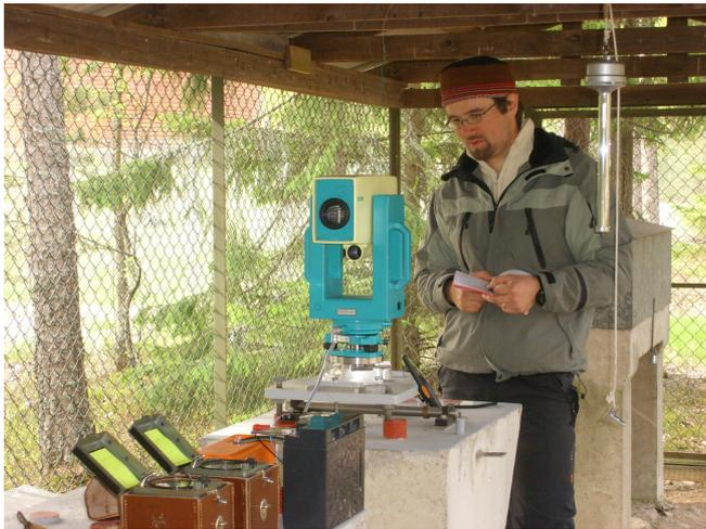
Fig. 4. Calibration of Kern ME5000 EDM instrument at the Väisälä-type Nummela Standard Baseline.
