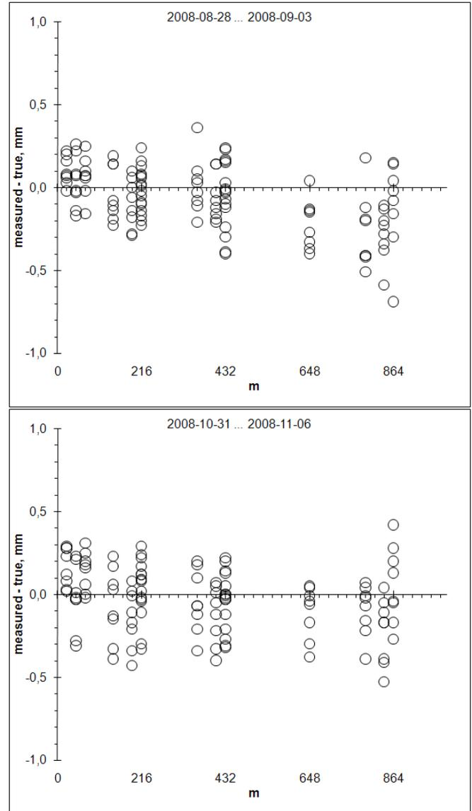
Fig. 5. Scale correction and additive constant of an EDM equipment are determined in calibrations before and after a scale transfer by comparing the measured values (after geometrical and velocity corrections) with true values from interference measurements. Here is an example of the calibrations at the Nummela Standard Baseline for scale transfers in autumn 2008.
