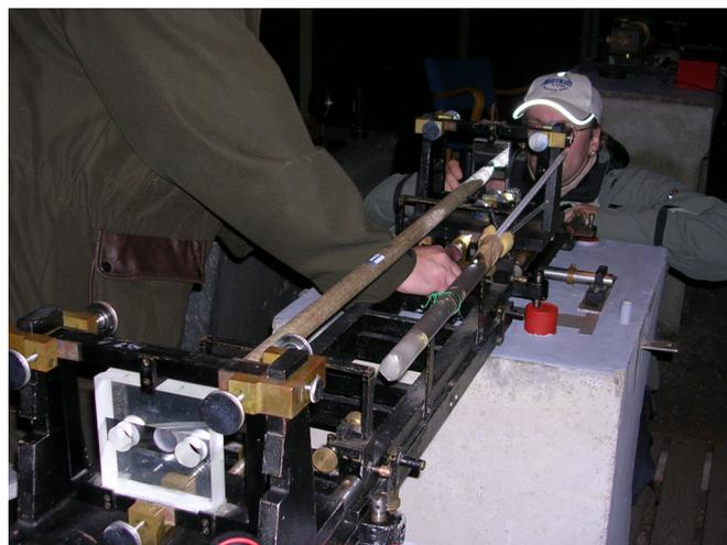
Fig. 3. The quartz metre no. VIII installed in the Väisälä interference comparator.
