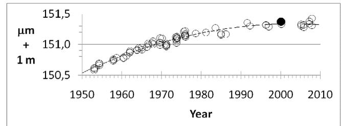
Fig. 1. Change of length of quartz metre no. VIII from comparisons at Tuorla. The filled circle is the latest absolute calibration. This quartz metre is always used in the Väisälä interference comparator at the Nummela Standard Baseline.
