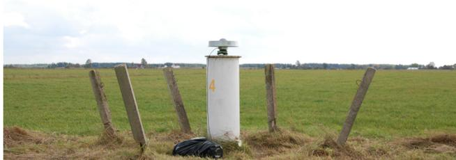
Fig. 6. The 7-pillar 1 320-m geodetic baseline and test field of the Vilnius Gediminas Technical University at Kyviškės in Lithuania are an optimal place also for testing of GPS equipment.
